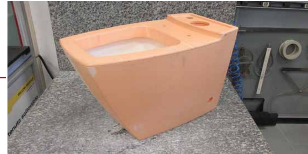
PROTOTYPE CAM DRILLING - 3D PRINTING / HYDRAULIC FUNCTIONALITY VALIDATION
